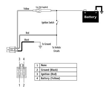
Figure 10. Wiring and pin outs for the 3-pin power harness.
